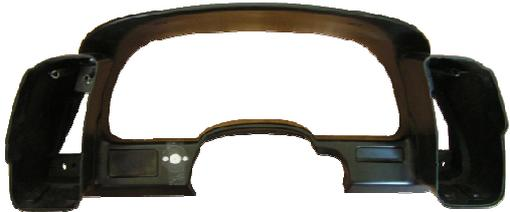
3. Drill holes. Outside holes use a 3/16" drill bit and centre hole uses a 1/2" drill bit
